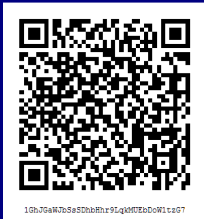
Figure 2: A Bitcoin address is the (double) hash of a public key. It has many different representations.
